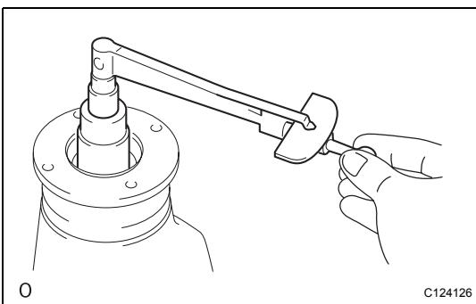
(c) Using a torque wrench, measure the preload.
