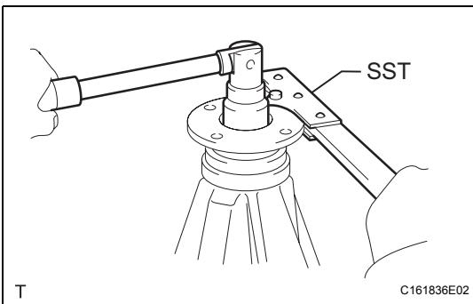
(d) Using SST to hold the companion flange in place, then slowly tighten the nut within the drive pinion preload adjustment range so that it reaches the specified drive pinion preload (at Starting).
