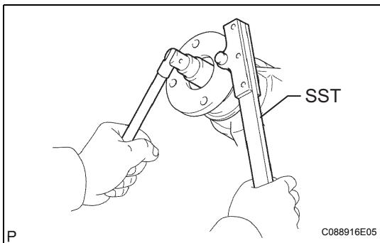
(b) Using SST to hold the companion flange in place, then slowly tighten the nut within the drive pinion preload adjustment range so that it reaches the specified drive pinion preload (at Starting).
