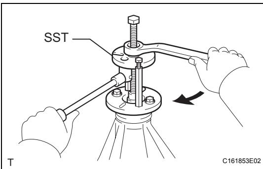
(c) Using SST, install the companion flange.
