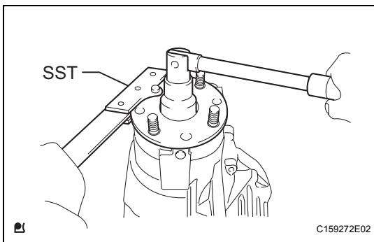
(c) Using SST to hold the companion flange in place, then slowly tighten the nut within the drive pinion preload adjustment range so that it reaches the specified drive pinion preload (at Starting).
