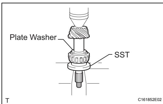
(b) Using SST and a press, press the rear bearing (inner race) into the drive pinion.
