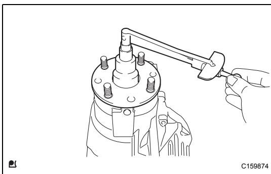
(c) Using a torque wrench, measure the preload of the backlash between the drive pinion and ring gear.
