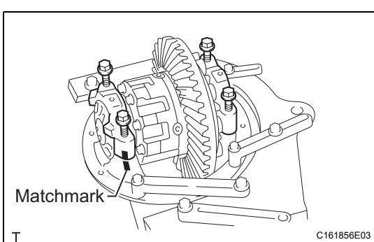
**12. INSPECT AND ADJUST DIFFERENTIAL RING GEAR BACKLASH**
