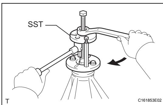
(b) Using SST, install the companion flange.
