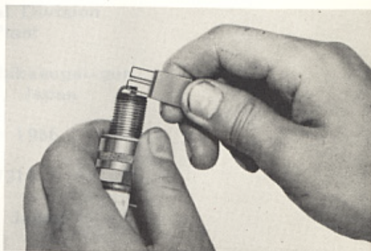
Fig.7-56 Adjusting Spark Plug Gap W0544
