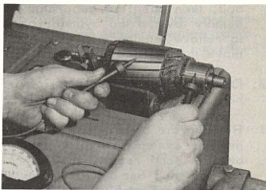
Fig.7-24 Testing Armature Commutator for Short W2744
