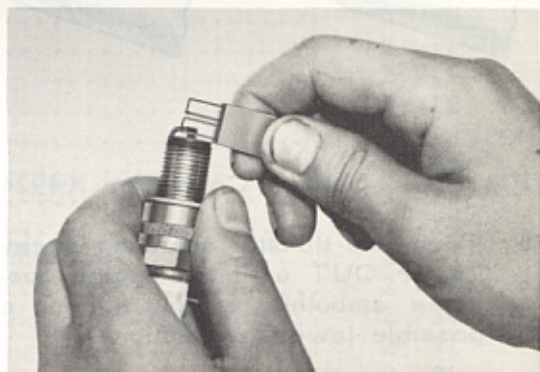
Fig.1-10 Adjusting Spark Plug Gap W0544
