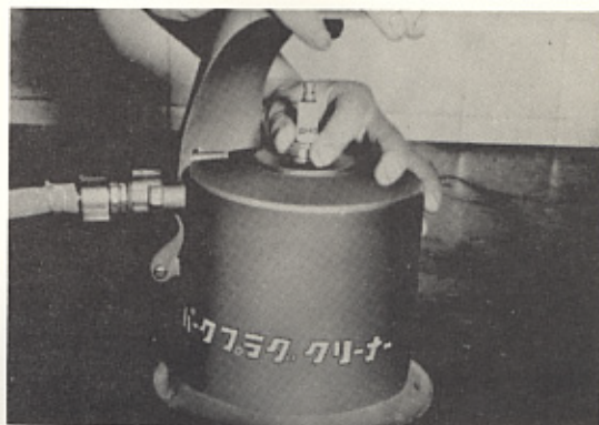
Fig.7-55 Cleaning Spark Plug W0543
